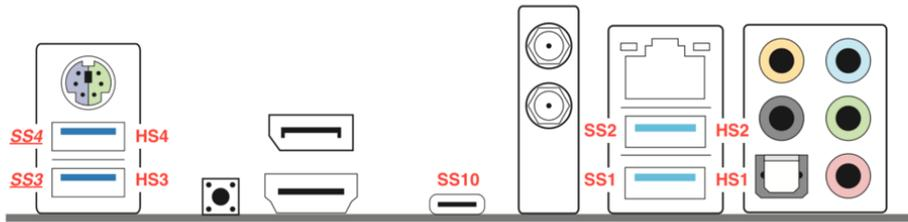
The front USB ports on the internal USB 3 header are SS5/HS5 and SS6/HS6. The port of the internal USB header is mapped to HS9, the internal Bluetooth module to HS10. In case the XHC0 controller is disabled, the ports 3/4 on the back I/O are USB 2 only.
