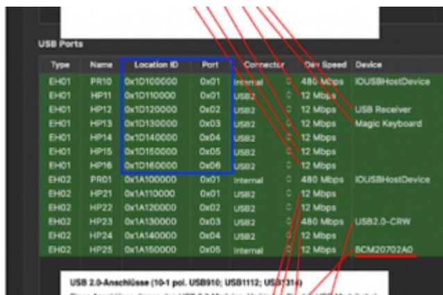
The screenshot shows a table titled "USB Ports" with the following columns: Type, Name, Location ID, Port, Connector, Dev Speed, and Device. The table lists 25 entries. Red arrows point to the "Port" column, highlighting that the value "0x01" is used for multiple entries (e.g., PR10, HP11, PR01, HP21, HP25), which is not unique. The device "BCM20702A0" is underlined in red.
