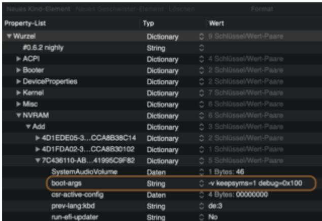
The screenshot shows the EFI configuration utility interface. The 'Property-List' table is expanded to show the 'boot-args' property, which is a String type with the value '-v keepsym=1 debug=0x100'. The 'boot-args' property is highlighted with a red circle.
